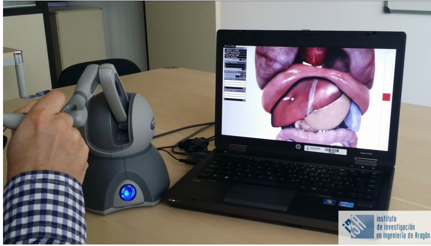
Figure 1: Surgical simulator. Prototype of surgical simulator developed by the authors. On the left, the haptic peripheral is shown.
