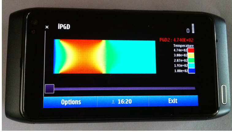
Figure 13. New optimal temperature field related to the reconfigured heating system.
