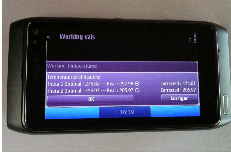
Figure 12. System reconfiguration by adjusting the temperature of the first heating device.
