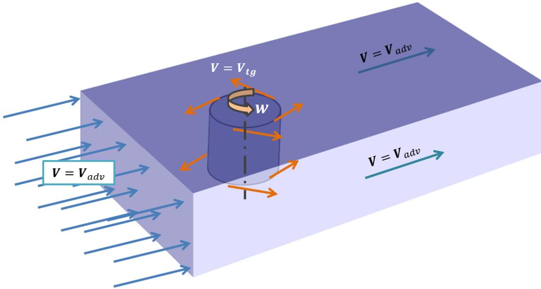
Figure 7: FSW kinematics model
