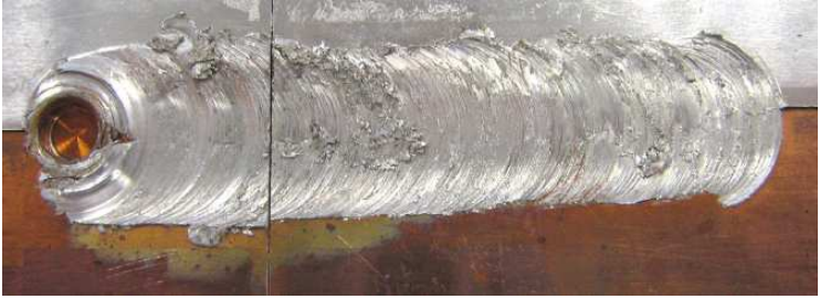
Fig. 15 Final result of the welding of two plates composed by Al 1050 and Cu b1.
