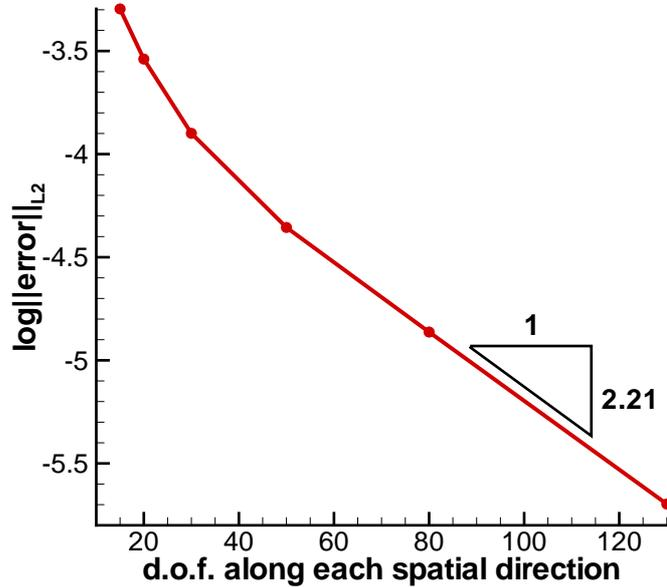
Figure 8. Solution convergence obtained by the proposed technique.
