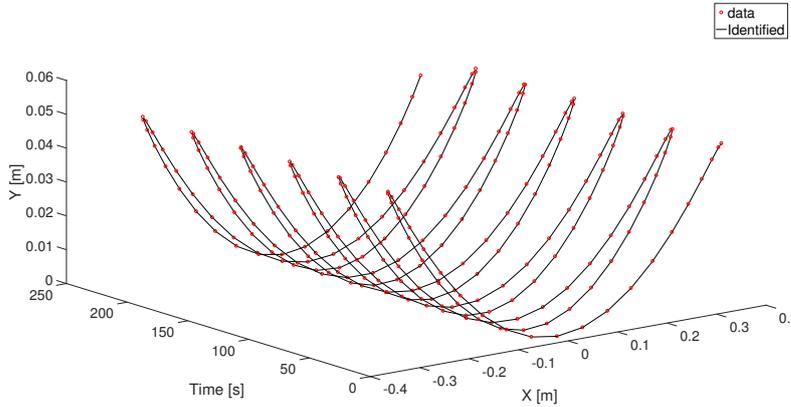
**Fig. 1** Results for the pendulum problem. Data (circles) vs. numerical integration of the identified system.
