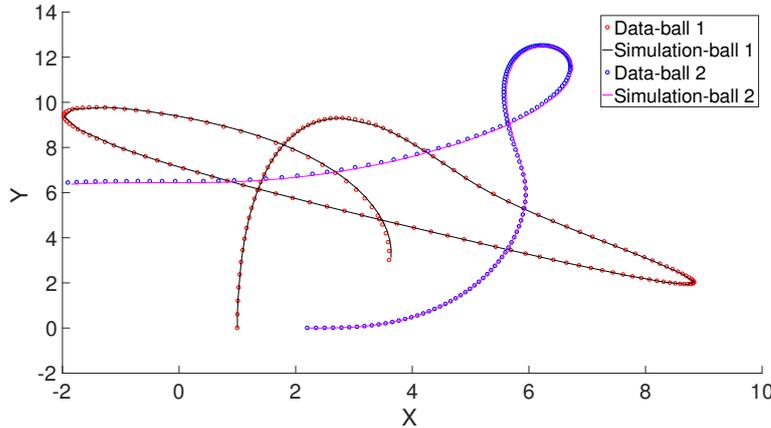
**Fig. 4** Results for the thermal pendulum problem. Trajectories of the two masses. Data (circles) vs. numerical integration of the identified system. Monolithic identification on sets of  $|\mathbf{z}^{\text{meas}}| = 34$  data points.
