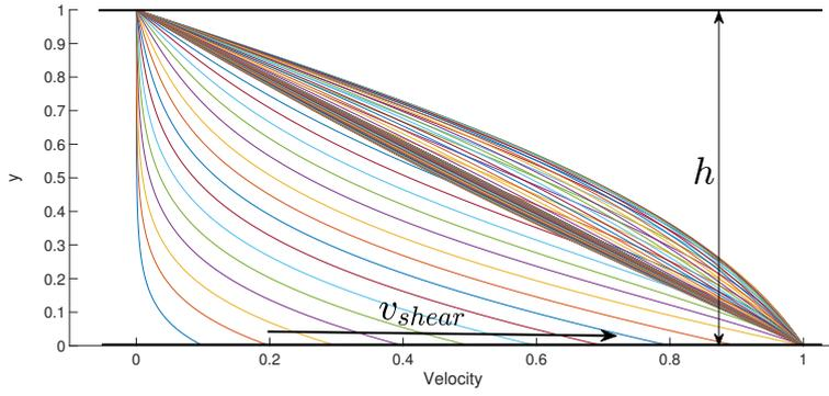
**Fig. 5** Velocity profile at every  $\Delta t = 0.01$  seconds ( $t \in (0, 1.5]$ ) for the startup of a Couette flow (shear flow between two plates, typical of a rheometer). In this case, velocity is imposed at the bottom plate, with  $h = 1.0$  and  $v_{shear} = 1.0$ . Notice the *overshoot* of the velocity profile just before the permanent regime (linear velocity profile).
