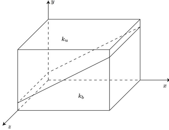
Figure 7: 3D case study involving a non-planar interface in the plate domain  $1 \times 10^{-3} \times 1$  (units in meters).
