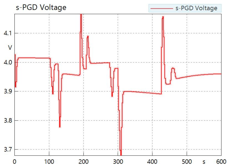
Fig. 26: Cell voltage predicted by the s-PGD model during the simulated itinerary.
